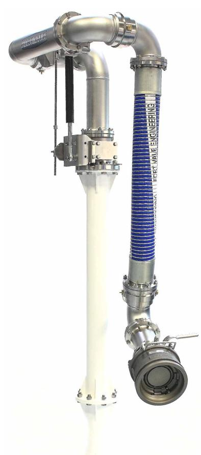
The Fort Vale 4" Safeload Loading Arm System consists of a combination of top-quality components, each with unique design features. Designed, manufactured and tested in-house, the Safeload System can be configured to produce a top or bottom loading arm solution.
