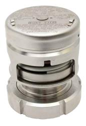
2½" Super Maxi Pressure/Vacuum Relief Valve with 80mm DIN11851 connection - Suitable for a pressure range of between 2 PSI to 75 PSI (0.14 Bar to 5.17 Bar) and a vacuum range of between 0.5"Hg to 24"Hg (0.02 Bar to 0.81 Bar). Contact parts manufactured in 316 stainless steel fitted with Fortyt seal (FEP encapsulated silicone O ring) as standard. Supplied complete with DIN 11851 fitting nut.
