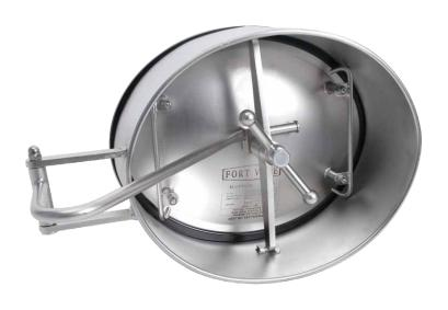
In/Out Oval Manlid Assembly with Deep Neckring - to suit Hygienic applications. 410mm x 508mm assembly with 200mm deep x 10mm thick neckring. Contact parts manufactured in 316 stainless steel polished to 180 grit. Cover fitted with vulcanised Blue Nitrile seal.
