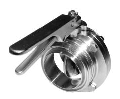
3" Concentric Disc Butterfly Valve - Suitable for hygienic applications. Inlet/outlet connections available include 3"BSP, 3"RJT, 3"Camlock, flanged and weld prepared. Single hand operation with TIR facility. Contact parts manufactured in 316 stainless steel fitted with Silicone seal as standard.
