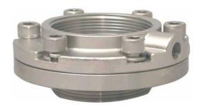
The burst disc adaptor assembly is designed to hold a 65mm burst disc between the tank and a  $2\frac{1}{2}$ " BSP relief valve. It is designed for use in conjunction with the Fort Vale manometer to monitor the integrity of the disc. (burst disc not included)
