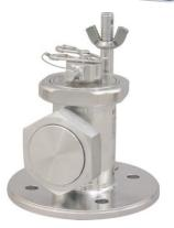
3" 3A Stamped Sanitary Milk Fitting Discharge Valve - 3" Bevel outlet. Inlet flange drilled 4 holes Ø 0.71" equispaced on a 6.00" PCD. (3" ANSI 150). Contact parts manufactured in 316 stainless steel with EPDM main seal. Supplied with weatherproof cowl.
