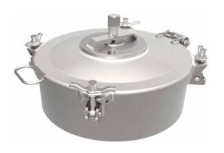
500mm Manlid Assembly with Flash Vacuum Vent - to suit Hygienic applications. 4 point fastening. 6mm thick x 150mm deep neckring. Manlid cover fitted with a flash vacuum vent set at 1"Hg (0.03 Bar). Neckring contact parts manufactured in 304 stainless steel. Manlid cover contact parts manufactured in 316 stainless steel. Fitted with stainless steel swingbolts with stainless steel handnuts. Seal supplied separately.
