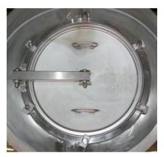
500mm Side Entry Manlid Assembly - suitable for Milk Tankers. Cover with cross arm and 6 point fastening with clamp system. 60mm deep neckring. Contact parts manufactured in 304 stainless steel. Fitted with a sweet white rubber seal. (FDA compliant)
