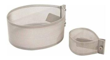
Clamped gauze rings are available for our 1",  $1\frac{1}{2}$ ",  $2\frac{1}{2}$ ", 65mm and 80mm relief valves. They clamp around the body ports and offer flame protection on valves with a vacuum setting of 0.21 Bar (6"Hg) and above. For valves with a vacuum setting of less then 0.21 Bar, a clamped gauze is often fitted to offer dust protection.
