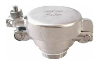
2"BSP Highflow Milk Breather Vent Valve - has a male screw connection and a hinged cap, enabling easy removal of the cap or the complete valve for inspection, cleaning and seal replacement. The cap can be opened by releasing the swingbolt. The valve has a food-grade silicone membrane seal which allows passage of air under pressure or vacuum conditions whilst preventing escape of liquid product during transit. Contact parts manufactured in 316 stainless steel.
