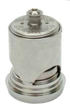
1½" Twinact Relief Valve with 50mm DIN11851 connection - Suitable for a pressure range of between 1 - 64 PSI (0.07 - 4.41 Bar) and a vacuum range of between 0.5" - 28" Hg (0.02 - 0.94 bar). Contact parts manufactured in 316 stainless steel fitted with Fortyt (FEP encapsulated silicone O ring) seals as standard. Complete with manual vent button.
