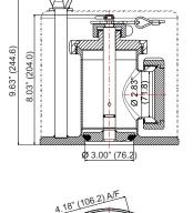
4 HOLES Ø 0.71" (18.0) EQUI-SPACED ON A 6.00" (152.4) PCD
