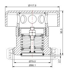
2" Vacuum Only Uniact Relief Valve with 65mm DIN11851 connection - Suitable for a vacuum range of between 0.5"Hg and 24"Hg (0.02 Bar and 0.81 Bar). Single-acting valve - vacuum relief only. Contact parts manufactured in 316 stainless steel fitted with Fortyt seal (FEP encapsulated silicone O ring) as standard. Supplied with stainless steel gauzed cap. 65mm DIN 11851 nut supplied separately.
