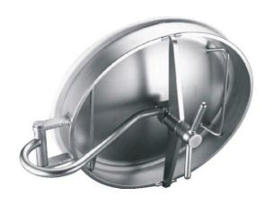
In-Out Oval Manlid Assembly - opens into the tank vessel, the cover may then be rotated to swing out through the manway. The manlid is operated using a double arm handnut and incorporates a cross arm to clamp and seal the cover on closure. Internal tank pressure enhances sealing performance. Contact parts manufactured in 316 stainless steel polished to 180 grit. Fitted with sweet white rubber seal as standard. Left hand operation.
