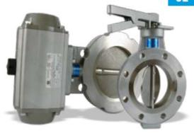
Rugged bulk solid version · Continuous shaft for optimum power transmission · Available with manual, pneumatic or electric operation · Nominal pipe sizes possible between DN 50 - DN 600 · Available as connecting part or end fitting version · Annular body: aluminium EN-AC 46200 · Standard materials inner parts: steel 1.0038 and stainless steel 1.4301 · Seal materials: NBR, EPDM, FPM, AU, MVQ, CSM and metal sealing
