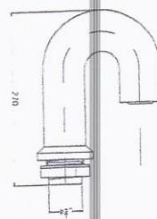
2" Diameter cuvered vent pipe in polyethylene
